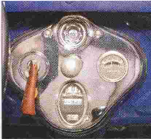
CLUSTER: The Model A driver had more information than ever before at his fingertips. By 1930, the dash cluster included gauges for measuring fuel, amperes, oil pressure, mileage, and trip mileage.
